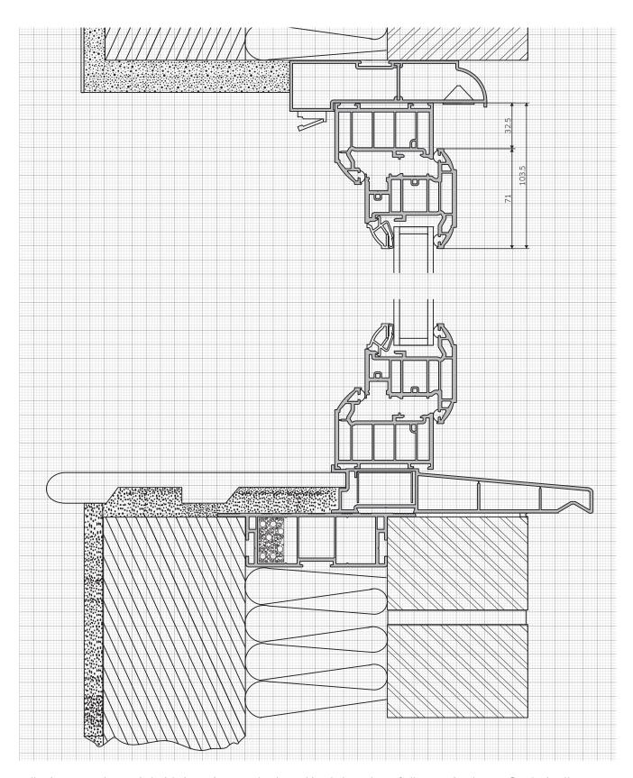
Following recent changes in legislation to improve the thermal insulation values of all properties the Duraflex Cavity Closer in being re-assessed to the new IP8/08 regulation. This will require insulation to be inserted in all cases. Please refer to the updated manual and bulletins to ensure compliance with regulations, contact our Technical Department for more information.
